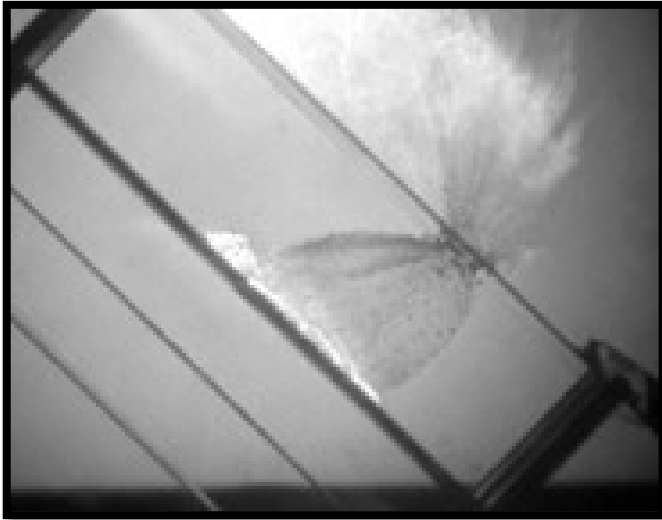
Figure 1: Hypervelocity impact test result at 7.2km/s
